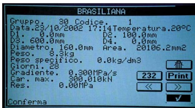
Screen showing the data of a tensile splitting test following the Standards UNI 6135.
