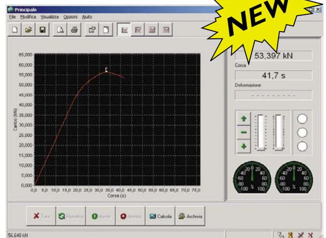
C109-12 Graphic example on Tensile Splitting Test.
