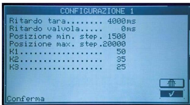
Personalisation of the working parameters of the machine in the advanced configuration menu protected by a password and restricted to the service engineers.
