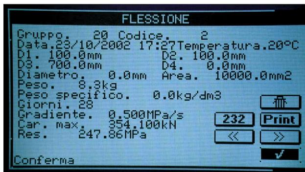
Screen showing the data of a flexure test.
