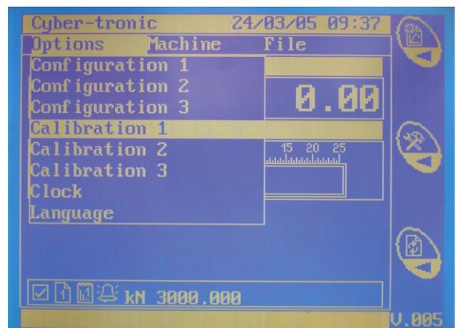
4 • Calibration menu up to 3 channels (3 testing frames) with its memorisation in the file.
