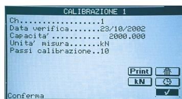
Checking screen of channel one calibration status (available on Cybertronic and Servotronic models)
