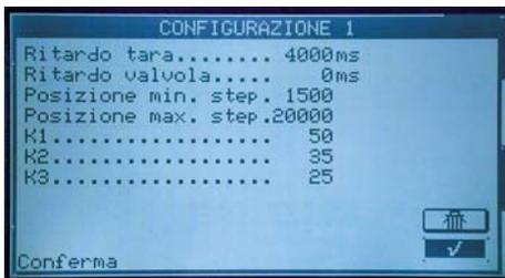
Personalisation of the working parameters of the machine in the advanced configuration menu, protected by a password and restricted to the service engineers (for Cybertronic and Servotronic models)
