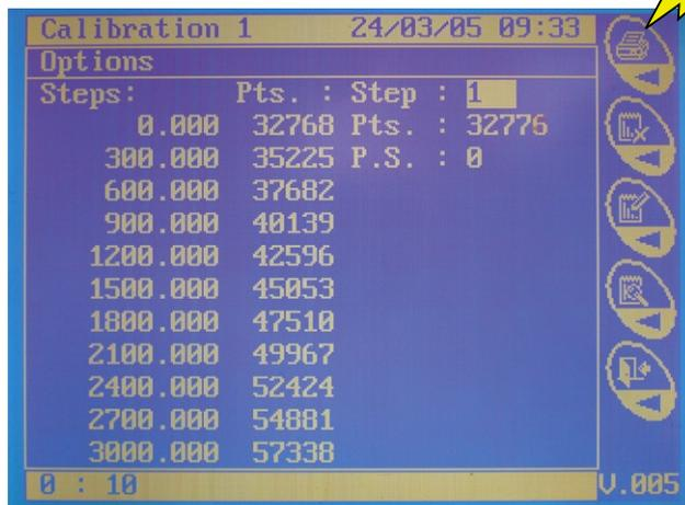
6 • Screen showing a calibration with confirmation of the reading lining points and file saving.
