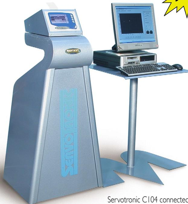
Servotronic C104 connected to a PC H009-01 with "Servonet" Licence C123 for the managing and the remote control of the test throughout all the phases.
